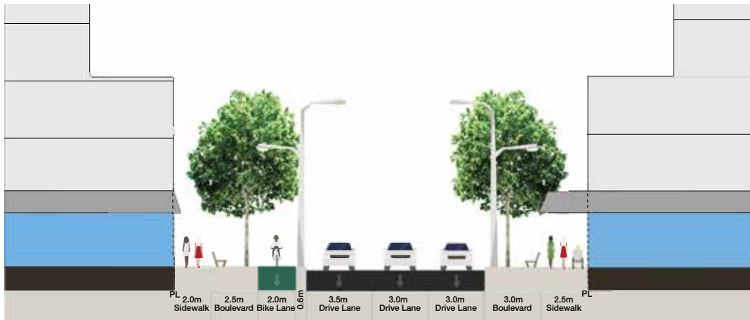
Figure 7.3: Conceptual cross section for Blanshard Street – One way (22 metres)
