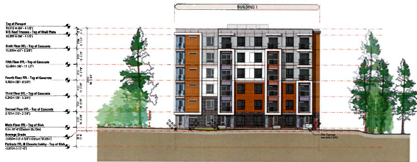
1 North Street Elevation (McCoy Road) A.11 Scale: 1:200
