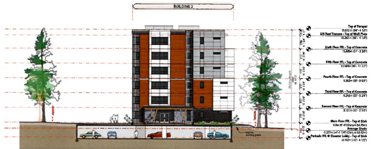
2 North Elevation (Courtyard) A.11 Scale: 1:200
