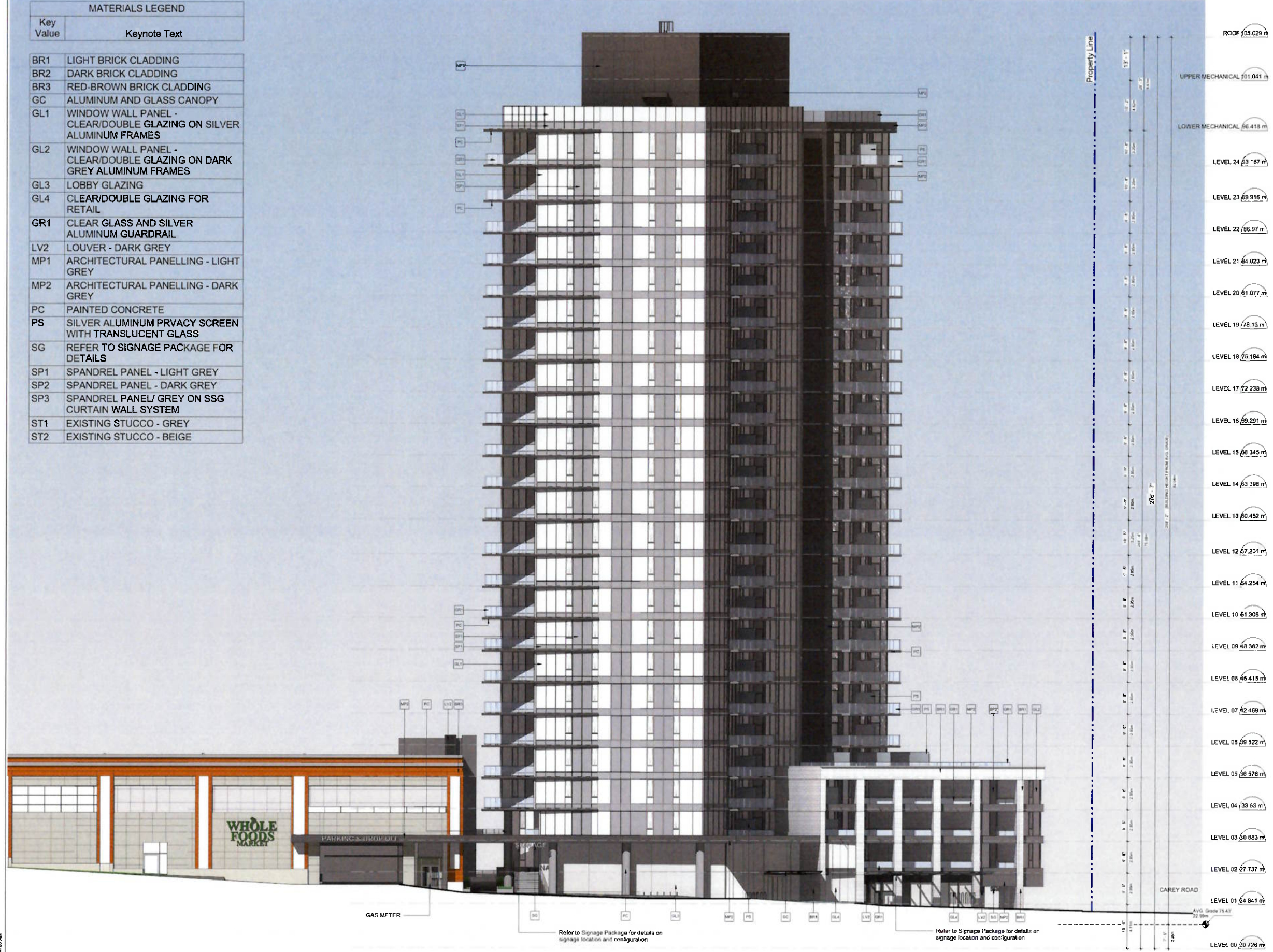
1 OVERALL NORTH ELEVATION - RAVINE WAY SCALE 3/32" = 1'-0"
