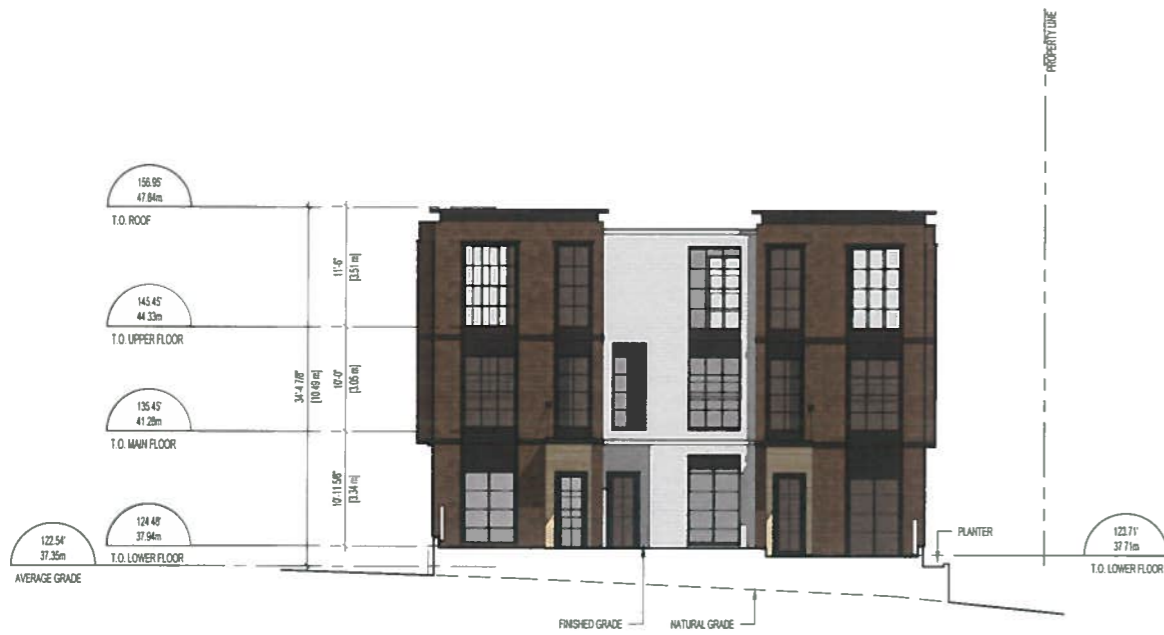
2 BUILDING D WEST ELEVATION 1/100
