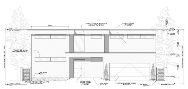
Figure 3: Proposed Front Elevation – viewed from Waring Place (from plans by Zebra Design)
