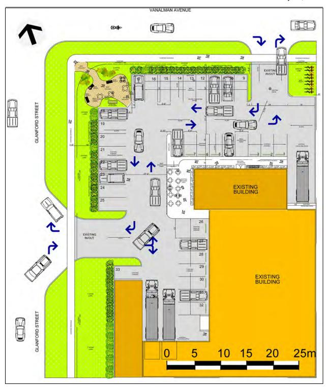
Figure 3: Proposed Parking Layout (from Plans by Fusion Design)
