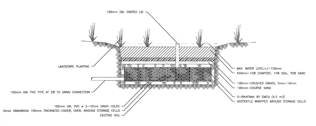
Figure 4: RAIN GARDEN TREATMENT/DETENTION - DETAIL
