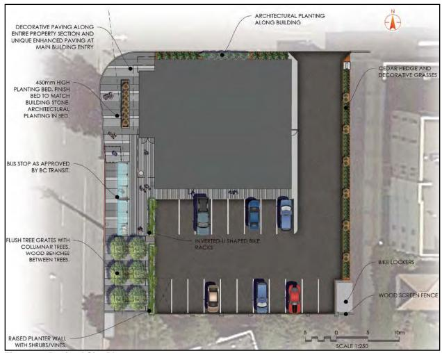
Figure 3: Revised Site Plan
