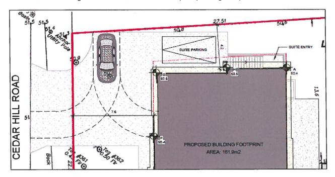
Figure 1: Vehicle Movement -Turning Radius (Provided by Ryan Hoyt Designs Inc.)
