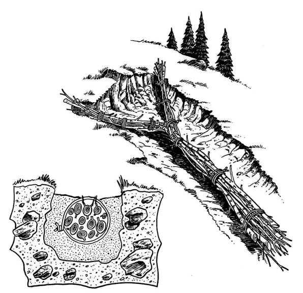
**Figure 2.** Live pole drains are bundles of cuttings that provide a preferred flow path for soil moisture.
