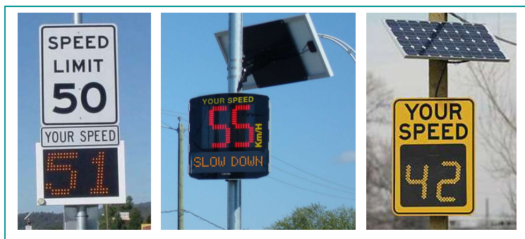
Figure 14 – Examples of Speed Reader Boards
