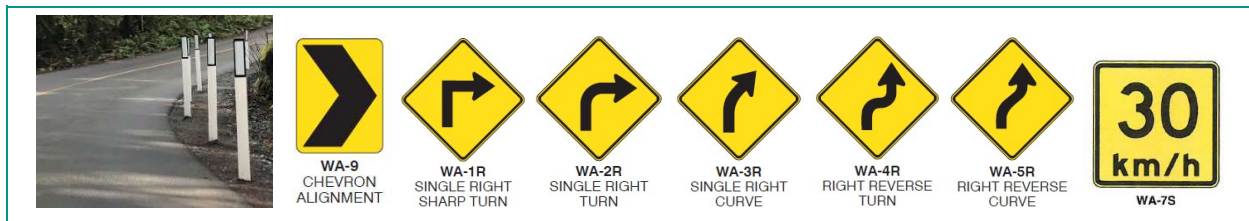
Figure 13 – Potential Signage at Roadway Curves
